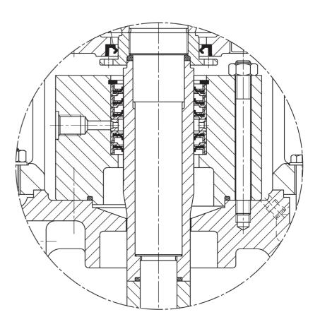
determined by the closing force of the pre-stressed sealing lips; usually 1.5 bar are sufficient.
