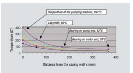
Temperature curve of casing wall and bearing support (ambient temperature: 15-20 °C)
