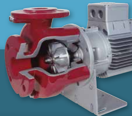
Extreme wear resistant: Type FB Recessed impeller pump for highly contaminated media
