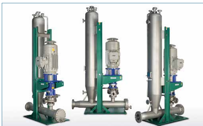
Fig. 2: Special centrifugal pump using the V-AN process: The pumping medium (hydrocarbon) is at its steam point. Feed rate: 120 to max. 132 m 3 /h Delivery height: 75 m Pump is operated at n=3000 rpm.
